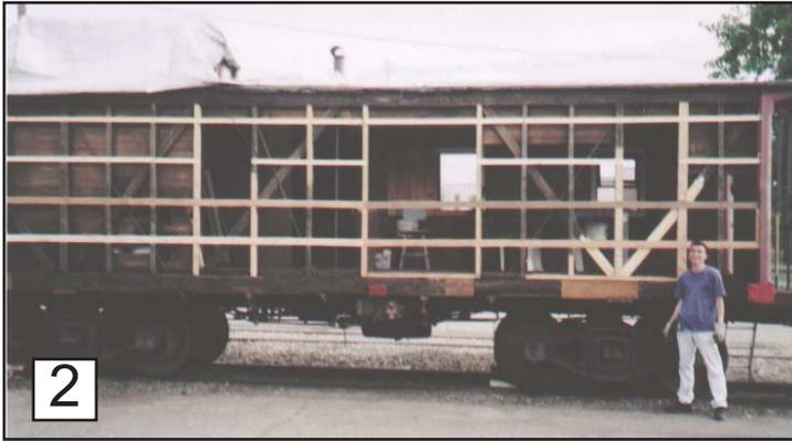
frames were fabricated by John Fegley, and installed in the window openings. A photo and explanation of the difficulties in completing the center window are in the "Little Red Caboose" article in the September 2006 issue of *The Railyard Local*.
