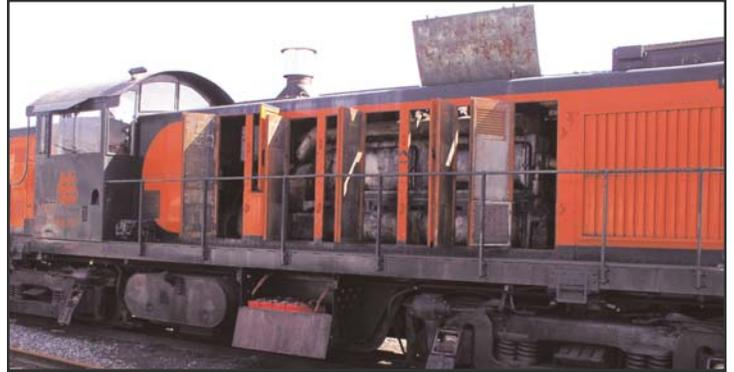
After the winter, checking on the RS1 diesel locomotive to see what work needs to be done before running it again.
