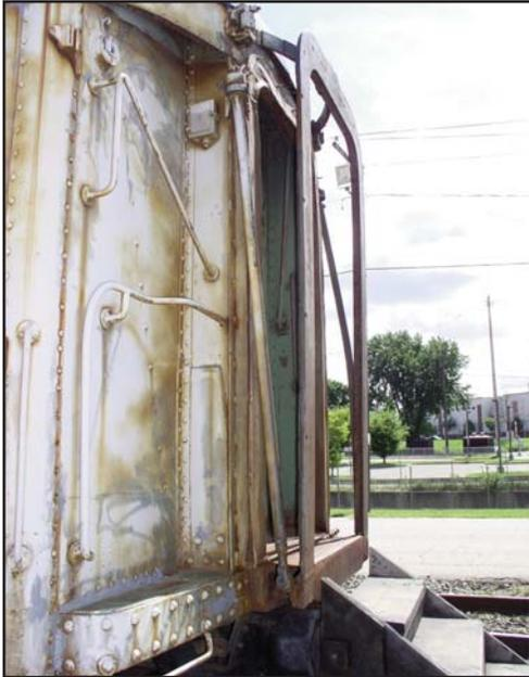
At left, one of the ends of the RPO car with the diaphragm removed. Photo above right, shows Bill Britt using an electric wire brush tool to clean corrosion off the window sills on the south side of the car. The same method was used to prepare the sides of the car for coating. What an amazing transformation!
