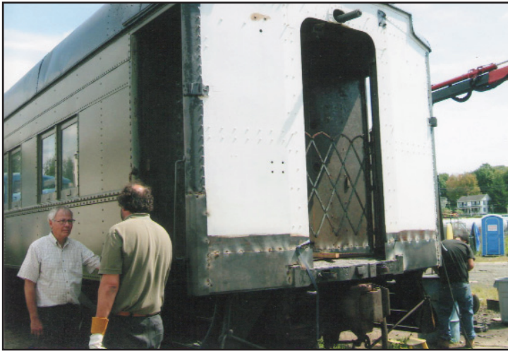
Top l., Art and Edelman's Metalworks, Inc. employee discussing reinstallation of diaphragm(r.); below l., hoisting diaphragm into place. Below r., finished forward right side, diaphragm reinstalled. Below, forward left side before and after patching; photos just above and below by Carolyn Taylor; others by Bill Britt, Project Leader
